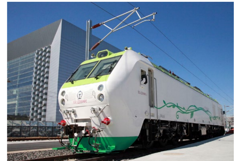
Permanent magnet direct-drive electric locomotive
